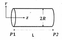
Q4: (a) Derive the expression for one-dimensional Non-steady state diffusion of carbon in a semi-infinite rod of mild steel with initial carbon concentration  $C_i$  and concentration of carburizing atmosphere  $C_o$ . The diffusivity of carbon in iron at temperature T can be assumed as  $D_{c,Fe}$ . (6 marks)
